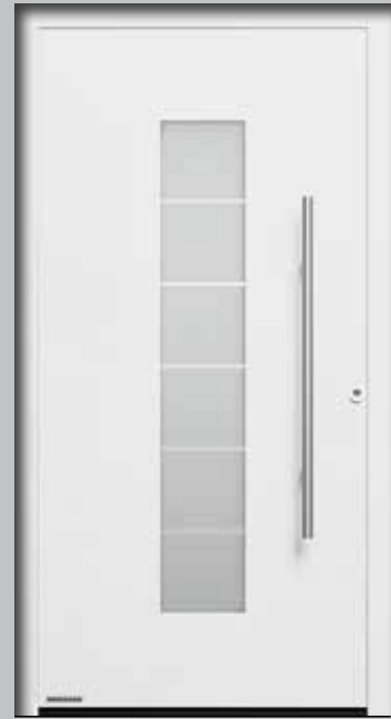
Style 504 Stainless steel handle HOE 500, matt float design glass with 5 clear horizontal stripes, triple thermal insulation glass, U_D -value up to approx. 0.9 \text{ W}/(\text{m}^2\cdot\text{K})^*
