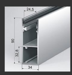
The guide sections are extruded 90mm x 3mm aluminium complete with wind lock recess, neoprene brush seals internally and externally.
